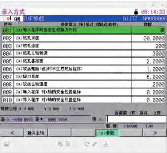
Parameter setting before CAD generated to G code.
